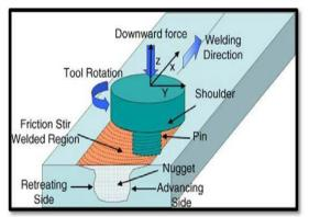
Fig. 1. Schematic diagram of FSW
