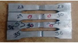
Fig. 5. Fractured specimens of weld joints formed from Hexagonal tip tool
